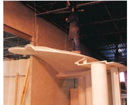
A FACTORY MOCK UP OF A COMPLEX DOME (NOTE THE MAN STANDING ON TOP)
